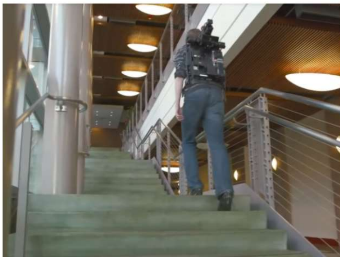
Wearable devices such as Indoor Reality's backpack offers a portable solution for mapping interior spaces. Image retrieved from a video by Berkeley Engineering.
