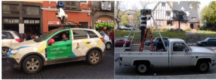
Google's Street View Car (Left) and the Ground-Based Data Acquisition System (Right) first developed by Berkeley's Video and Image Processing Laboratory.
